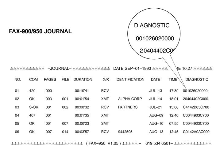
Figure 5-7. Identifying the Diagnostic Code in a FAX-900/950 Journal
