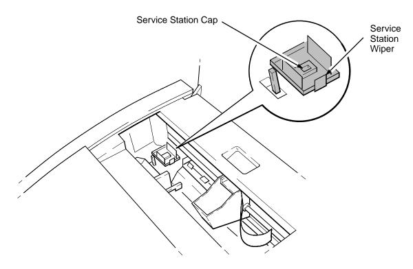
Figure 3-18. Cleaning the Service Station Cap and Wiper on the HP FAX-700 and FAX-750
