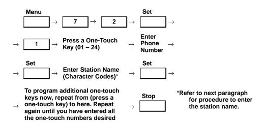
**Entering your station name (15 characters maximum).** Use the one-touch keypad to enter the alphabetic characters. Use the Dial/Space button for inserting spaces between characters. The default for the FAX-950 one-touch keypad is that the lower character of each key will be printed to the message window until P4 is pressed to print upper characters. Once P4 is pressed, upper characters will be printed until P4 is pressed again or power is cycled.
