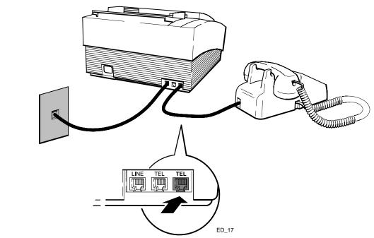
Figure 2-40. Connection the HP FAX-700 and FAX-750 to the Telephone
