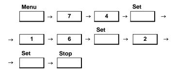
In the Telephone Answering Machine Interface Mode, the answering machine attached to the HP FAX-900 or FAX-950 will answer all incoming calls and begin the outgoing message you recorded on the answering machine tape. The HP FAX-900 or FAX-950 will not pick up the line. During the outgoing message, the fax machine will monitor the incoming line for a fax tone signal.
