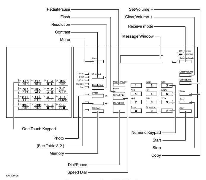
Figure 3-2. Control Panel (HP FAX-900)
