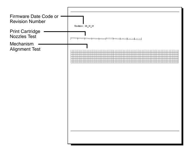
Figure 5-10. GPM Self-Test Pattern (Test Mode 0)
