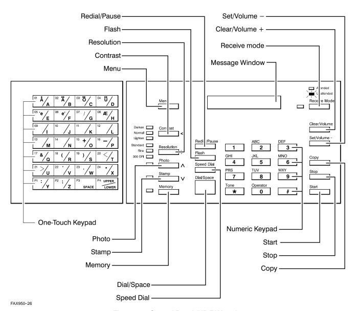
Figure 3-3. Control Panel (HP FAX-950)
