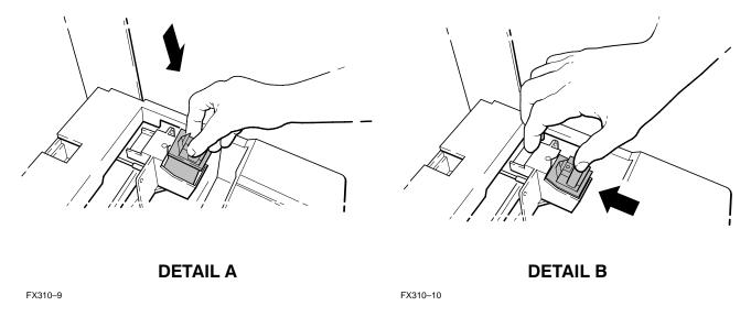
Figure 2-10. Print Cartridge Installation on the HP FAX-900 and FAX-950
