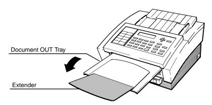
Figure 2-25. Extending the HP FAX-700 and FAX-750 Document OUT Tray
