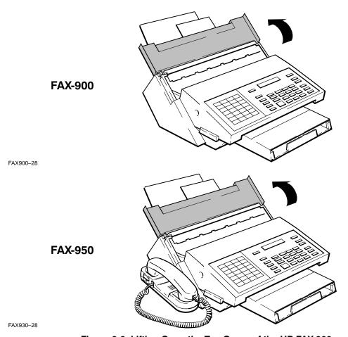
Figure 3-9. Lifting Open the Top Cover of the HP FAX-900 and FAX-950
