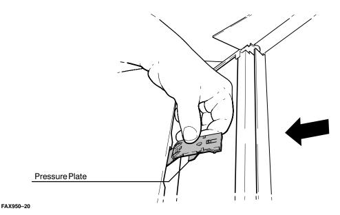
Figure 2-33. Installing the Replacement Paper Separator
