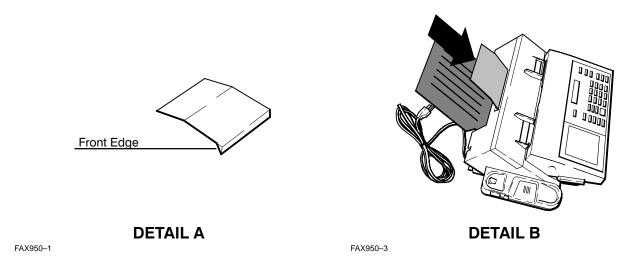
Figure 2-28. Installing the HP FAX-900 and FAX-950 Document IN Tray (HP FAX-950 Shown)
