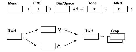
Note: It is possible to enter a code from Table 5-32 in order to initialize RAM data instead of pressing  $\land$  or  $\lor$  to select the data to be initialized. The fax machine will immediately initialize after the last digit of the code is pressed.
