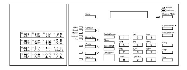
Figure 2-6. Control Panel (HP FAX-900)
