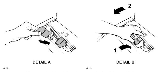
Figure 2-12. Installing the Print Cartridge on the HP FAX-700 and FAX-750
