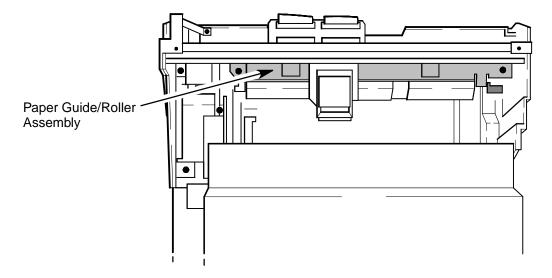
Figure 3-19. Cleaning the Paper Guide/Roller Assembly
