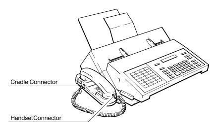
Figure 2-37. Installing the Handset in the HP FAX-950
