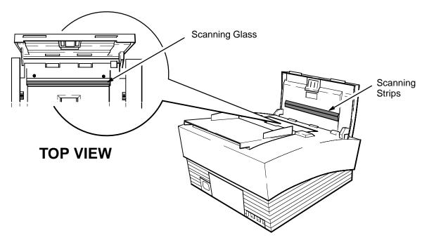
Figure 3-16. Wiping the Scanning Glass and Strips on the HP FAX-700 and FAX-750
