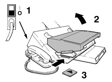
Figure 2-29. Installing the Expandable Memory Card
