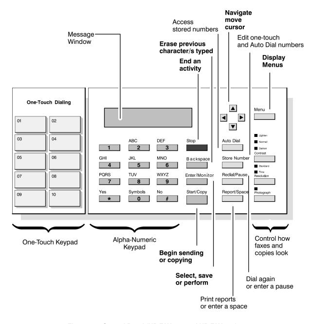
Figure 3-1. Control Panel (HP FAX-700 and HP FAX-750)
