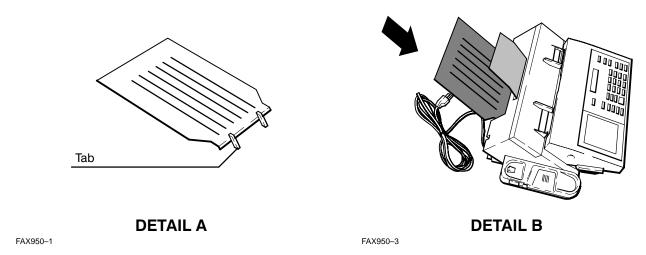
Figure 2-26. Installing the HP FAX-900 and FAX-950 Document OUT Tray (HP FAX-950 Shown)
