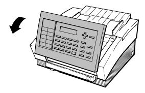
Figure 2-30. Lifting the ADF Door
