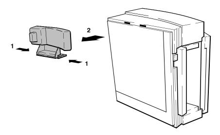
Figure 2-36. Removing the Handset Base
