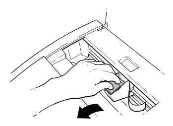
Figure 3-10. Moving the Cartridge Forward
