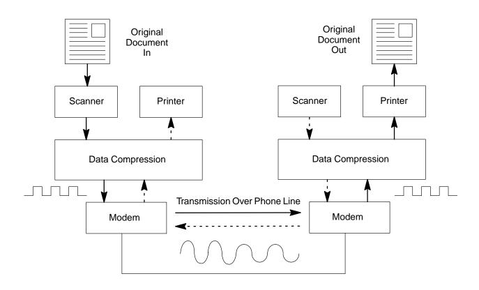
Figure 1-1. Simple Diagram of Transmission Between Fax Machines
