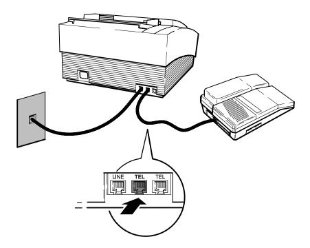
Figure 2-42. Connecting the HP FAX-700 to an Answering Machine
